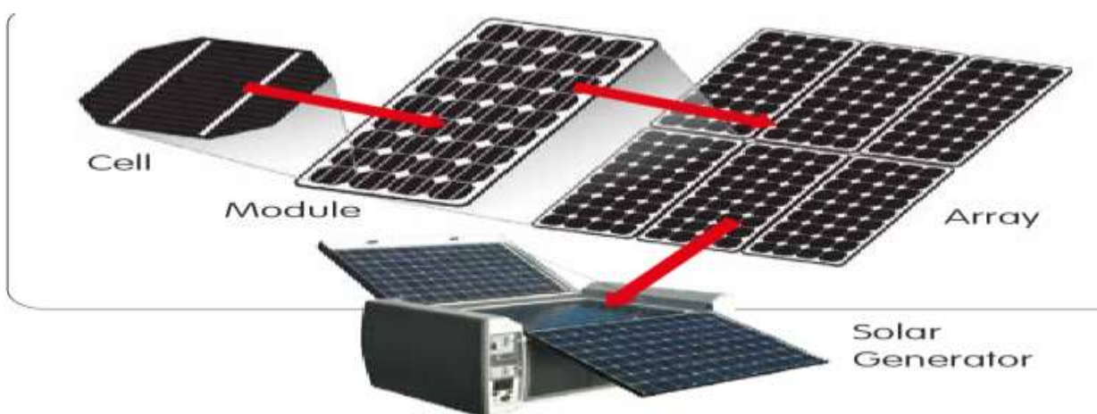
Figure 5.3 Solar cell, module, array and solar generator
